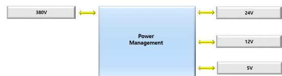
Fig. 8. Block diagram of the power unit of the complex microbial incubator.
