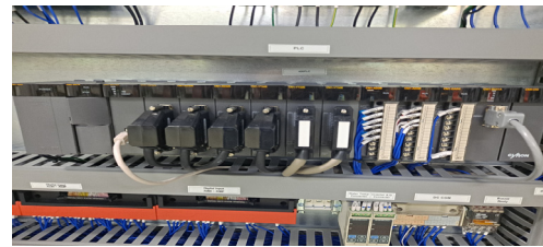
Fig. 7. Communication unit of the manufactured complex microbial incubator.
