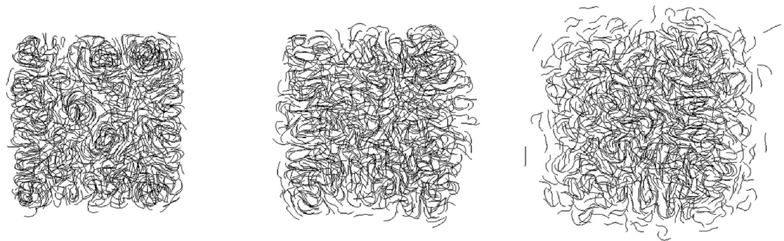
Figure 13. SPH-based turbulent flow simulation using the proposed Bitonic sort-based hashing for NNP queries. The simulation uses identical physical parameters and rendering settings as the baseline, while replacing only the hashing/sorting backend, enabling higher particle counts and improved performance without sacrificing visual fidelity.
