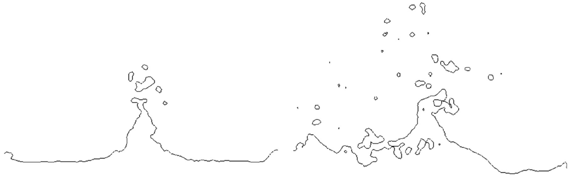
Figure 12. SPH surface reconstruction using the proposed Bitonic sort-based hashing for nearest-neighbor particle (NNP) queries. This example uses approximately 50,000 particles under the same simulation and rendering settings as the baseline, and demonstrates that acceleration of neighbor search does not degrade reconstruction quality.
